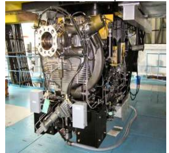
Stand for Testing the Fuelling Machine
